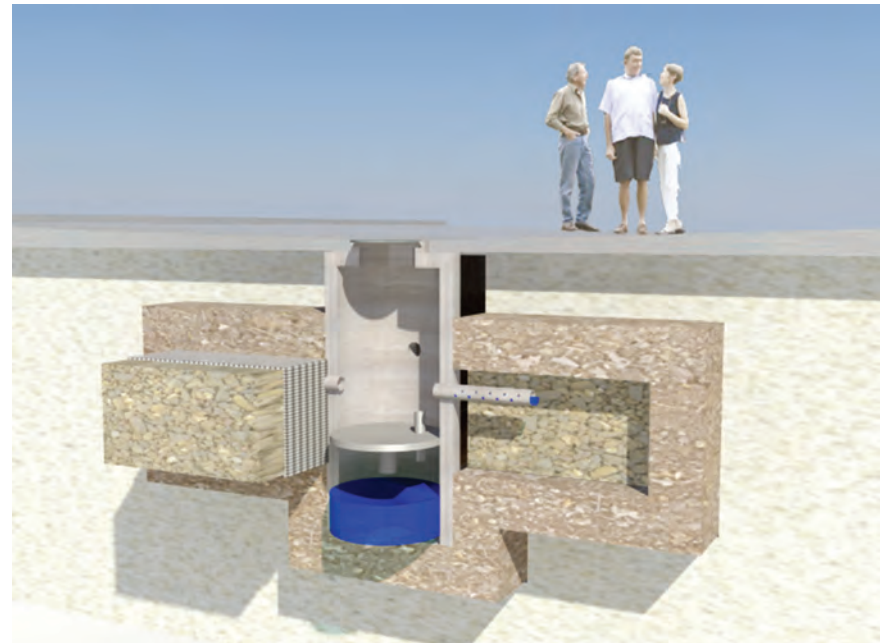
Figure 6.19. Section through a catch basin with oil and grit separator, combined with infiltration trenches. The runoff is conveyed to infiltration trenches that can be varied in length and storage capacity.
